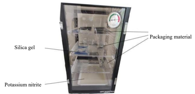
Figure 5. Accelerated Shelf Life Testing Set-Up According to ASTM.
