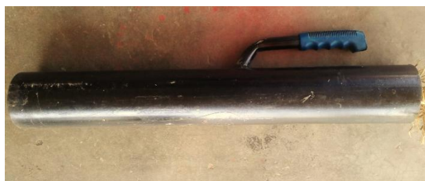
Figure 5. Fabricated combustion chamber of the smoker.
