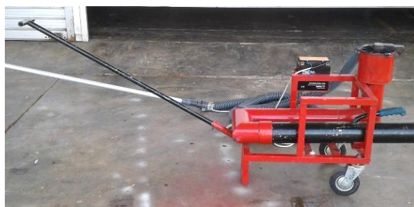
Figure 4. The mobile and height-adjustable smoker for giant honeybees.
