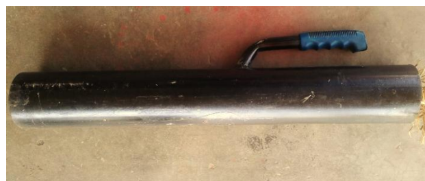
Figure 5. Fabricated combustion chamber of the smoker.
