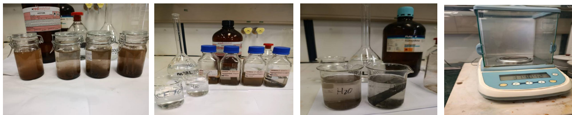
Figure 10. Coupons after 26 days of immersion in test solutions (with/without plant extracts) at 50 °C.
