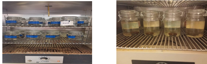
Figure 8. Coupons immersed in test solutions at 50 °C during the 26-day exposure period.
