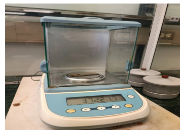
Figure 6. Initial preparation and weighing of coupons using a digital balance ( \pm 0.0001 mg).
