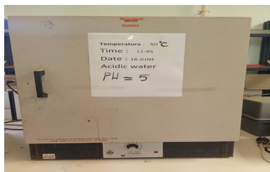
Figure 9. Oven used to maintain the coupons at 50 °C for 26 days during immersion in the inhibitor-containing solutions, simulating long-term exposure conditions.
