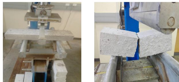
(a) Beam specimen on flexural machine beam before loading (b) Ultimate failure of a specimen due to flexural load
