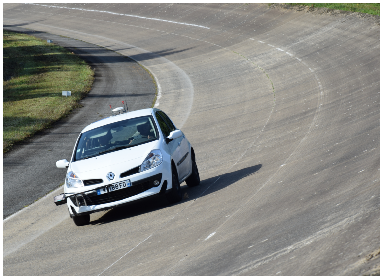
Figure 3. Test vehicle on the C_2 crossfall level trajectory.
