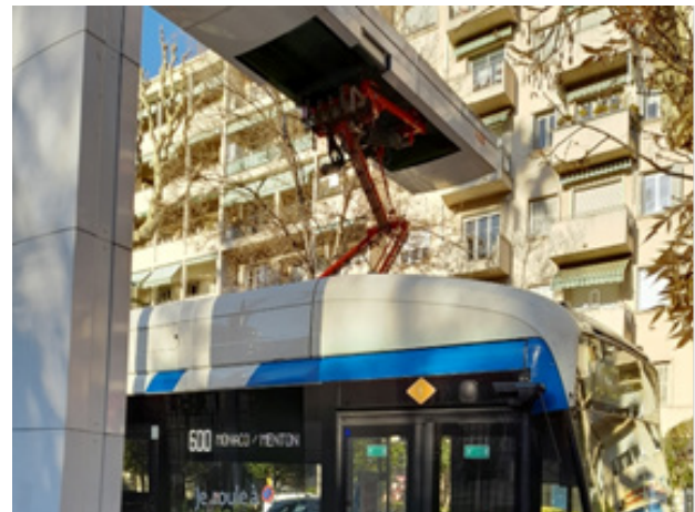
Figure 4. Bus using a rooftop charging device during the terminal break without passengers.
